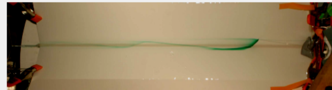
Figure 17: The "Ekman Helix" traced out by dye injected in the bottom boundary layer seen a) up the canyon and b) from above. The secondary circulation causes a particle to follow a helix like path down the canyon.
