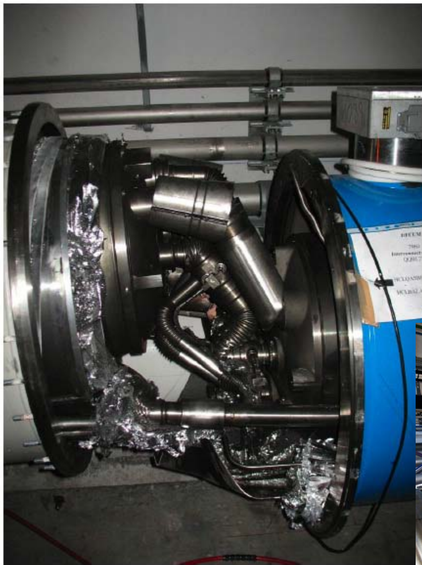
Geneva, 20 September 2006. During the final LHC sector (sector 3-4) an incident occurred at mid-day or a large helium leak into the tunnel.
